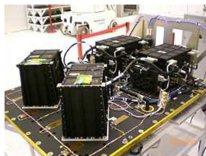
Figure 3 : Jason-3 Poseidon-3 Instrument
